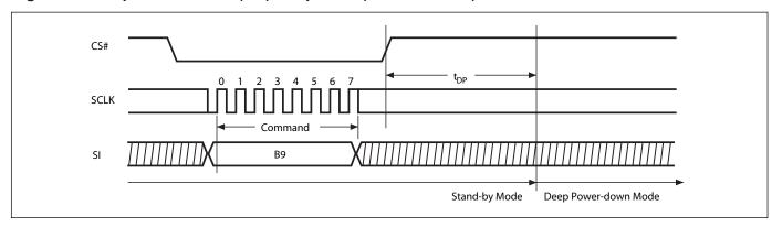
Figure 23. Release from Deep Power-down and Read Electronic Signature (RES) Sequence (Command AB)
