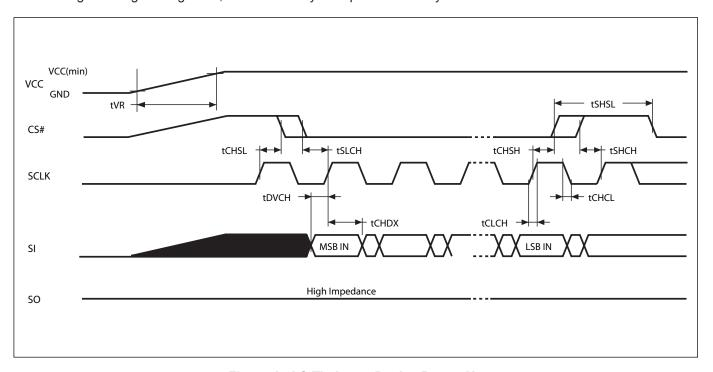
Figure A. AC Timing at Device Power-Up
