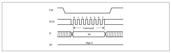
Figure 13. Read Identification (RDID) Sequence (Command 9F)
