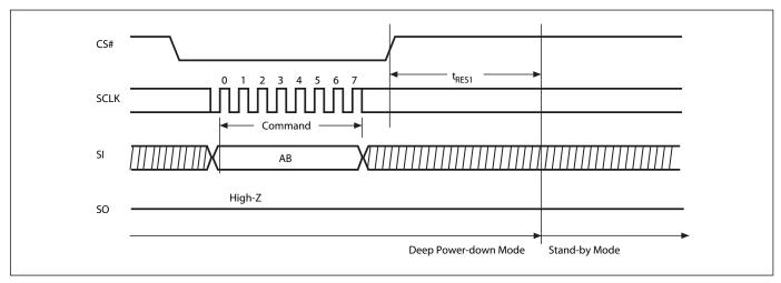
Figure 25. Read Electronic Manufacturer & Device ID (REMS) Sequence (Command 90)
