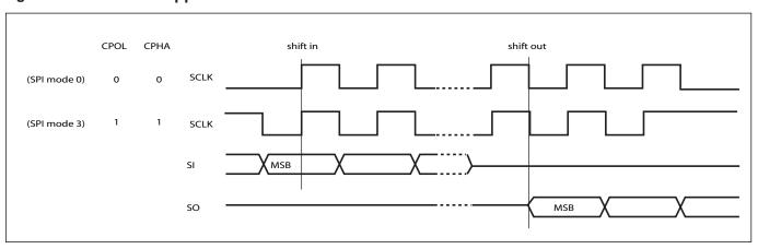
Figure 2. SPI Modes Supported
