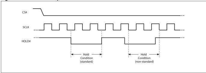
The Serial Data Output (SO) is high impedance, both Serial Data Input (SI) and Serial Clock (SCLK) are don't care during the HOLD operation. If Chip Select (CS#) drives high during HOLD operation, it will reset the internal logic of the device. To re-start communication with chip, the HOLD# must be at high and CS# must be at low.
